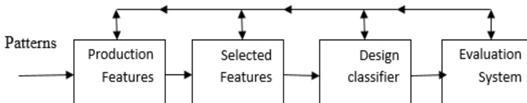
Fig. 1 The block diagram of the pattern recognition system
