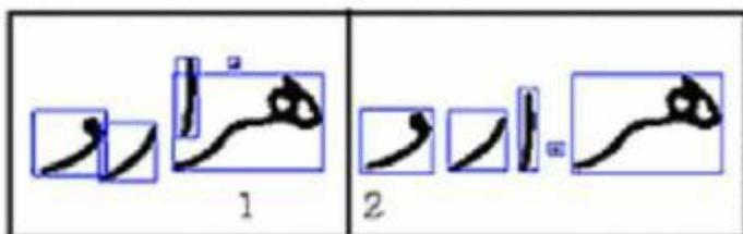
Fig. 9 sub character isolation by flood fill algorithm
