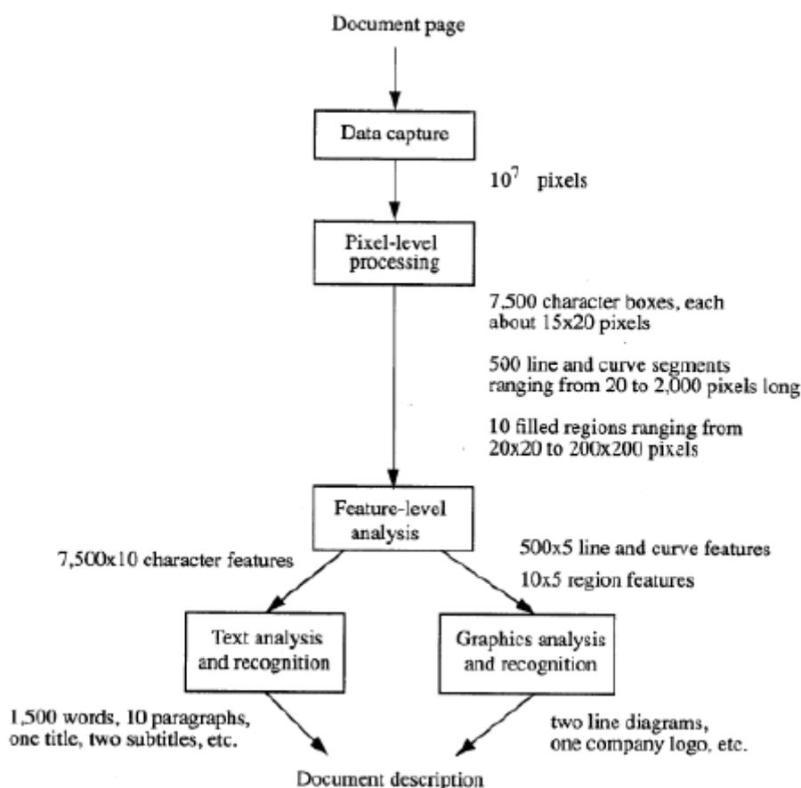
**Fig. 2 Block diagram of recognition system**
