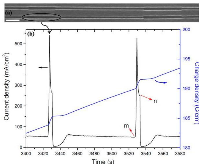
**Figure 2.** Current density and charge density–time curve of the sample made in the phosphoric/oxalic acid mixture containing 0.1M phosphoric acid at 170V and the corresponding cross-sectional SEM micrograph (The scale size is 300 nm).
