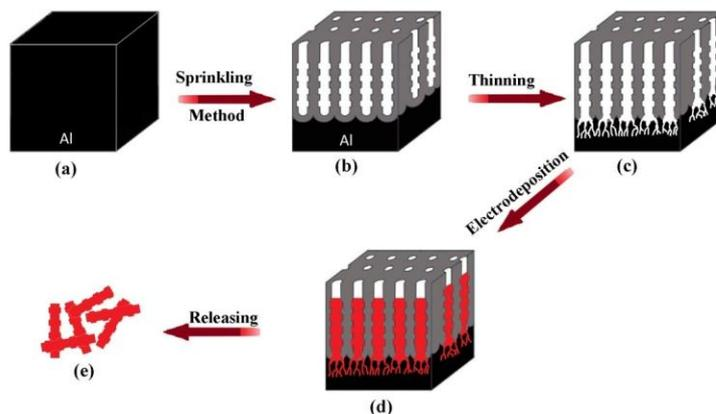
**Figure 1.** Schematic diagram describing the fabrication steps of diameter modulated metallic nanowire arrays based on porous anodic alumina template.
