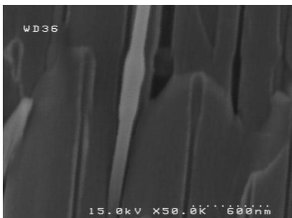
**Figure 4.** Cross section SEM micrograph of diameter–modulated Cobalt nanowire inside the alumina pore.
