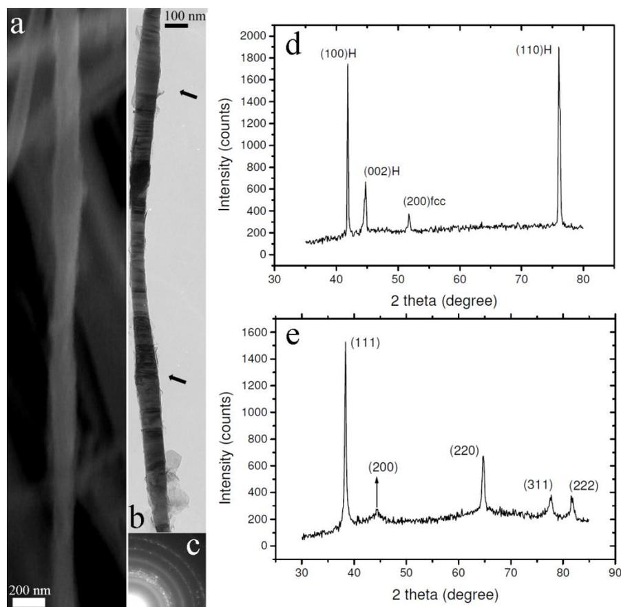
**Figure 5.** SEM image of diameter–modulated Ag nanowire after removal of AAO template. (b) TEM image of diameter–modulated Co nanowire and (c) corresponding ED pattern. (d) and (e) X-ray diffraction patterns of Co and Ag nanowires array respectively.
