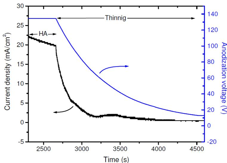
**Figure 3.** Current density, Voltage–time curve of sample during thinning process
