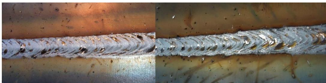
Figure (4a) welding with ratio of 80:20      Figure (4b) welding with ratio of 60:40
