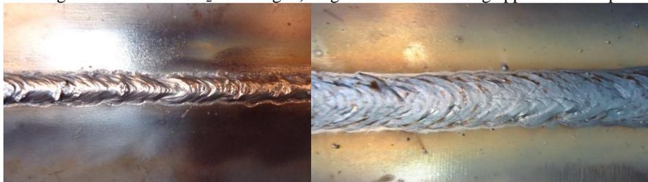
Figure (3 a) welding with pure CO<sub>2</sub>      Figure (3b) welding with pure Argon
