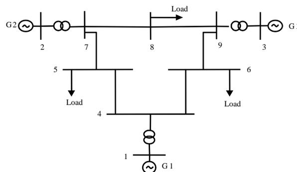
**Fig. 3. Three-machine nine-bus power system.**
