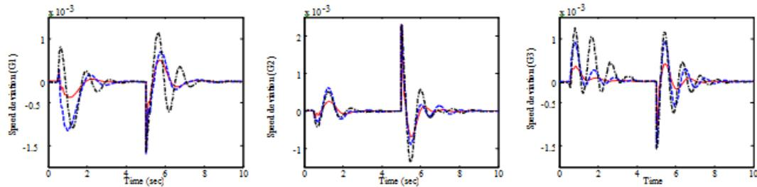
Fig8. System response under heavy loading in scenario II; Solid (IHBMOPSS), dash (PSOPSS), Dash-dotted (CPSS)
