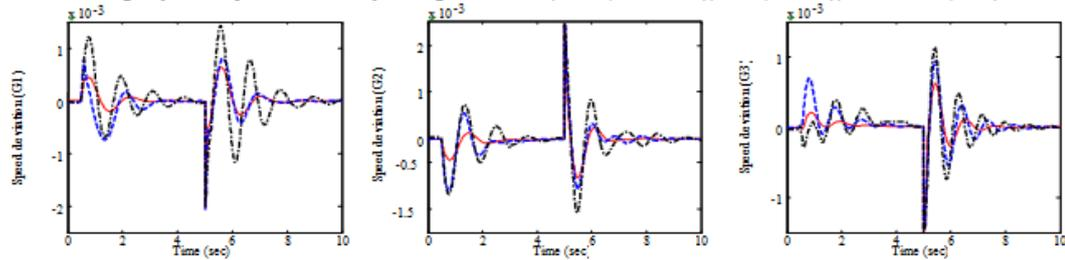
Fig9. System response under nominal loading in scenario II; Solid (IHBMOPSS), dash (PSOPSS), Dash-dotted (CPSS)
