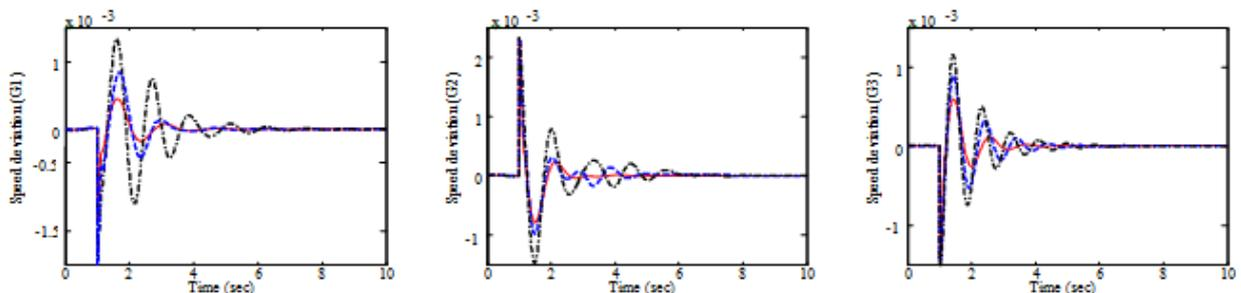
Fig5 - System response under nominal loading in scenario I; Solid (IHBMOPSS), dash (PSOPSS), Dash-dotted (CPSS)
