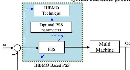
**Figure 4. The proposed IHBMO based PSS controller structure.**
