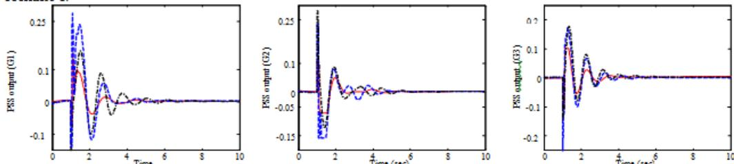
Fig 11. System response under heavy loading in scenario I; Solid (IHBMOPSS), dash (PSOPSS), Dash-dotted (CPSS)
