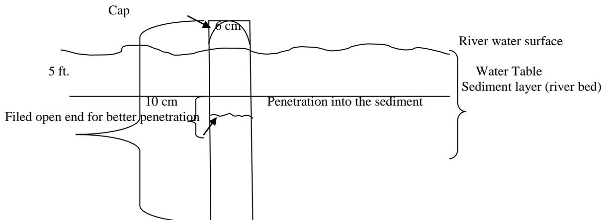
**Figure 1. A schematic representation of sampling with a corer. Also shown are the dimensions of the corer**
