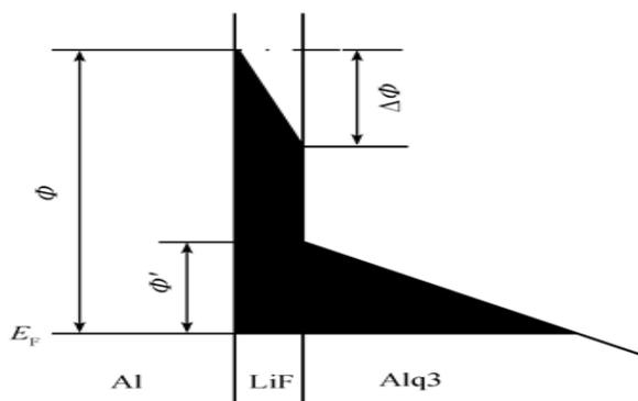
**Fig. 1: Schematic diagram of the tunneling model with a LiF buffer layer.**
