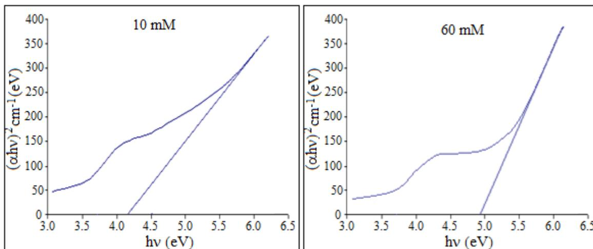
**Fig. 6** Tau's plot of ZnS:Mn nanoparticles with different concentration of ME
