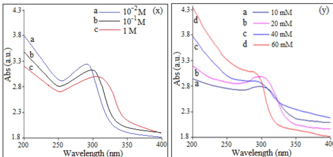
**Fig 4(x) Absorption spectra of ZnS:Mn samples with different molar concentration**
