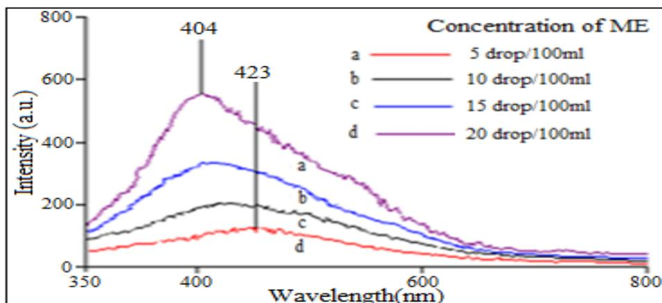
**Fig.8 PL spectra of ZnS nanocrystals with different concentration of ME**
