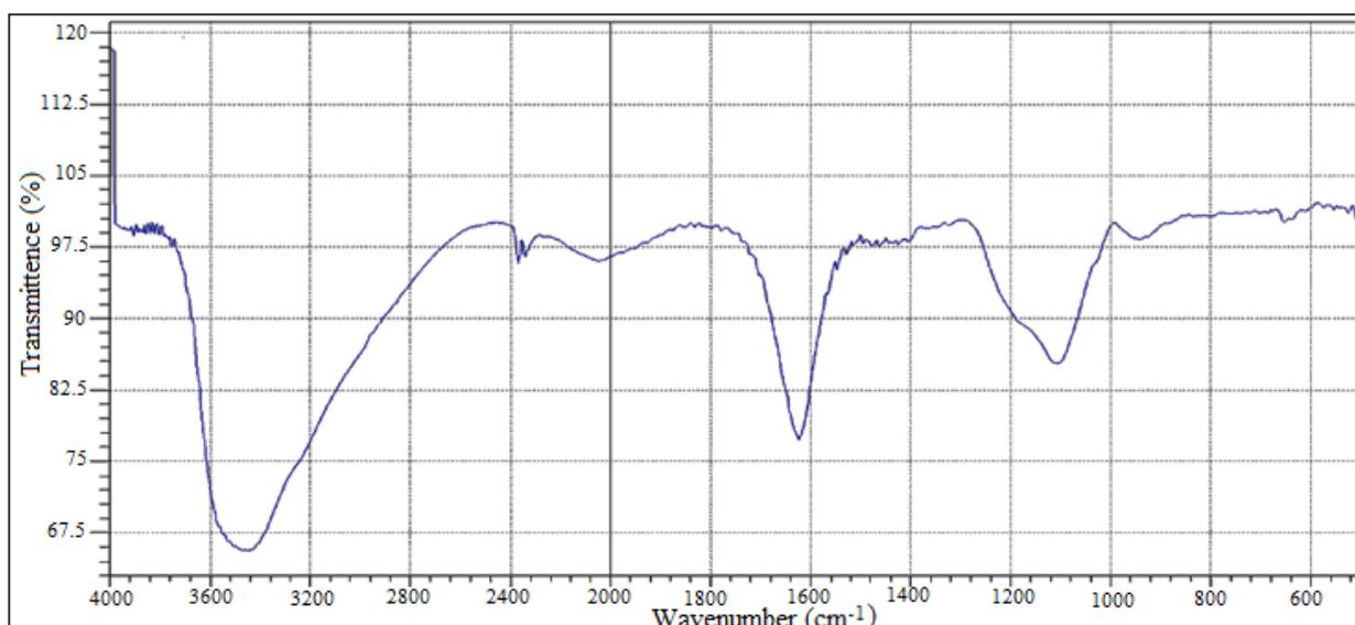
**Fig. 7 FTIR spectra of ZnS:Mn nanocrystals**
