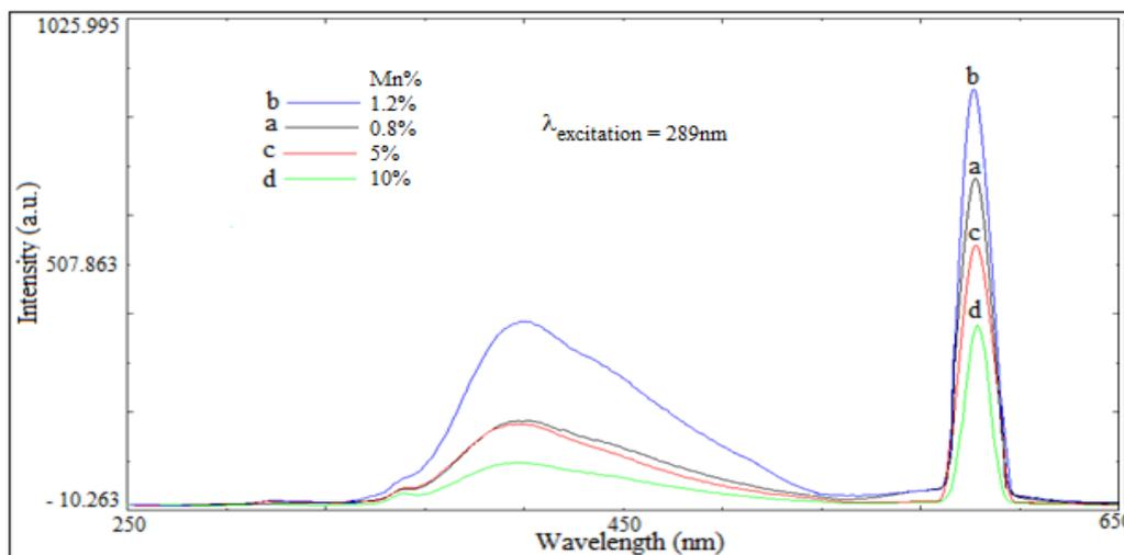
**Fig.9 Photoluminescence of ZnS:Mn nanocrystals with different concentration of Mn**
