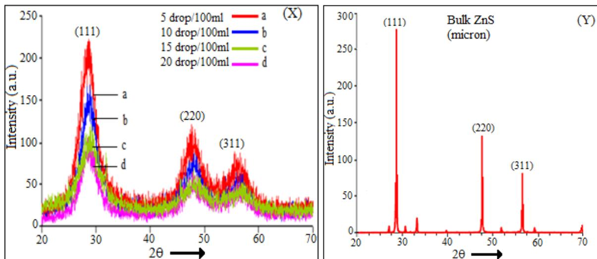
**Fig.1 XRD pattern of ZnS:Mn nanocrystals with different concentration of ME**
