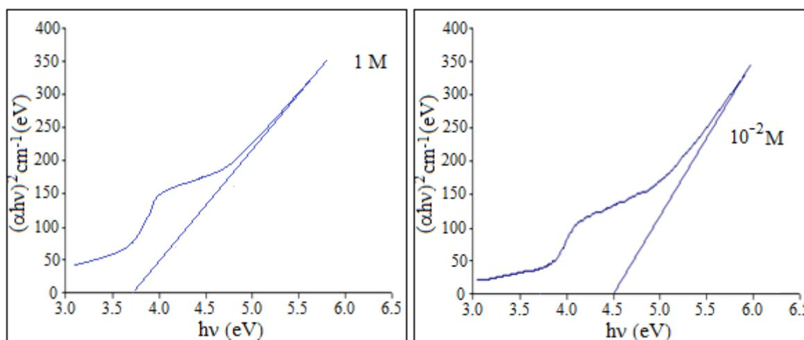
**Fig. 5 Tau's plot of ZnS:Mn nanoparticles with different molar concentration**
