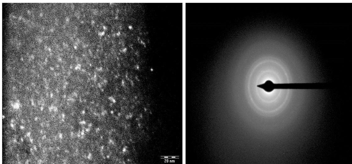
**Fig. 3 The Particle size measurement and SAED pattern of ZnS:Mn nanoparticles by TEM**
