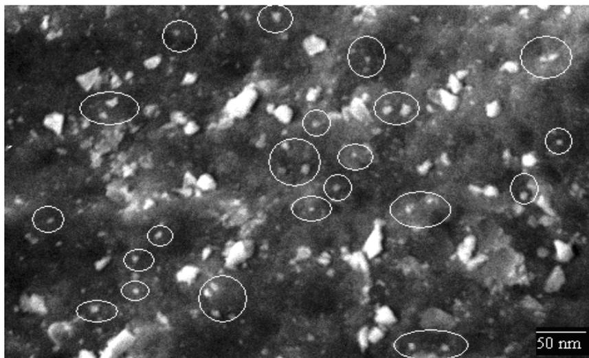
**Fig. 2 SEM photograph of ZnS:Mn nanocrystals**
