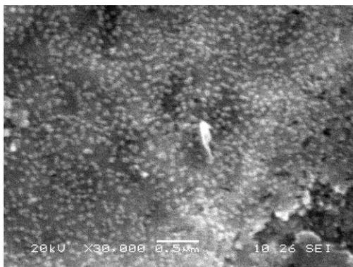
**Fig.3: SEM image of SnO<sub>2</sub> thin film**
