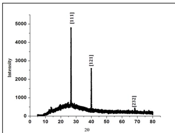
Figure-1. XRD Pattern for Molybdenum Oxide Spin Coated Thin Films.
