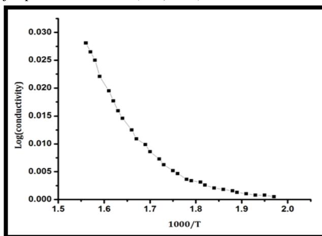
Figure-5. Arrhenius Plot of dc conductivity vs.  $1000/T$  of  $\text{MoO}_3$  Thin Films.
