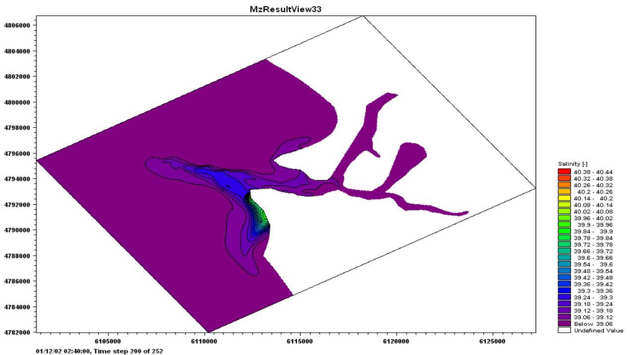
Figure 14. Simulation results in the depletion of salt, twelve days after the execution of the model
