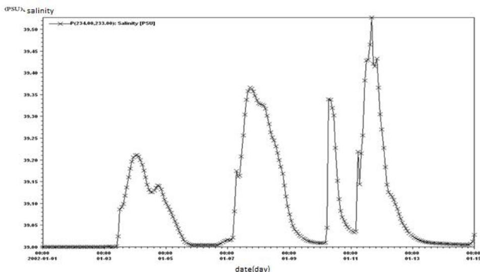
**Figure 12.** Simulation results in a radius of 200 meters of salt water for a period of 15 days from the time of discharge of effluent in simulation scenario 1 (a distance of 477 meters harvesting and hauling the prevailing conditions of wind and wave West)
