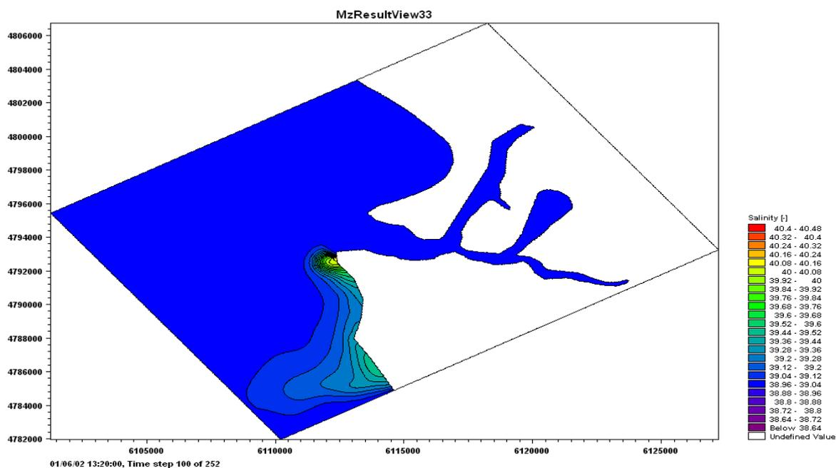
Figure 21. Simulated results of salinity at discharge, six days after the execution of the model
