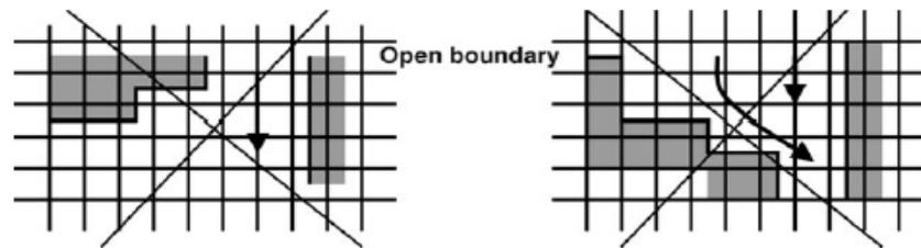
**Figure 2. Sudden contraction and expansion flow near an open boundary**
