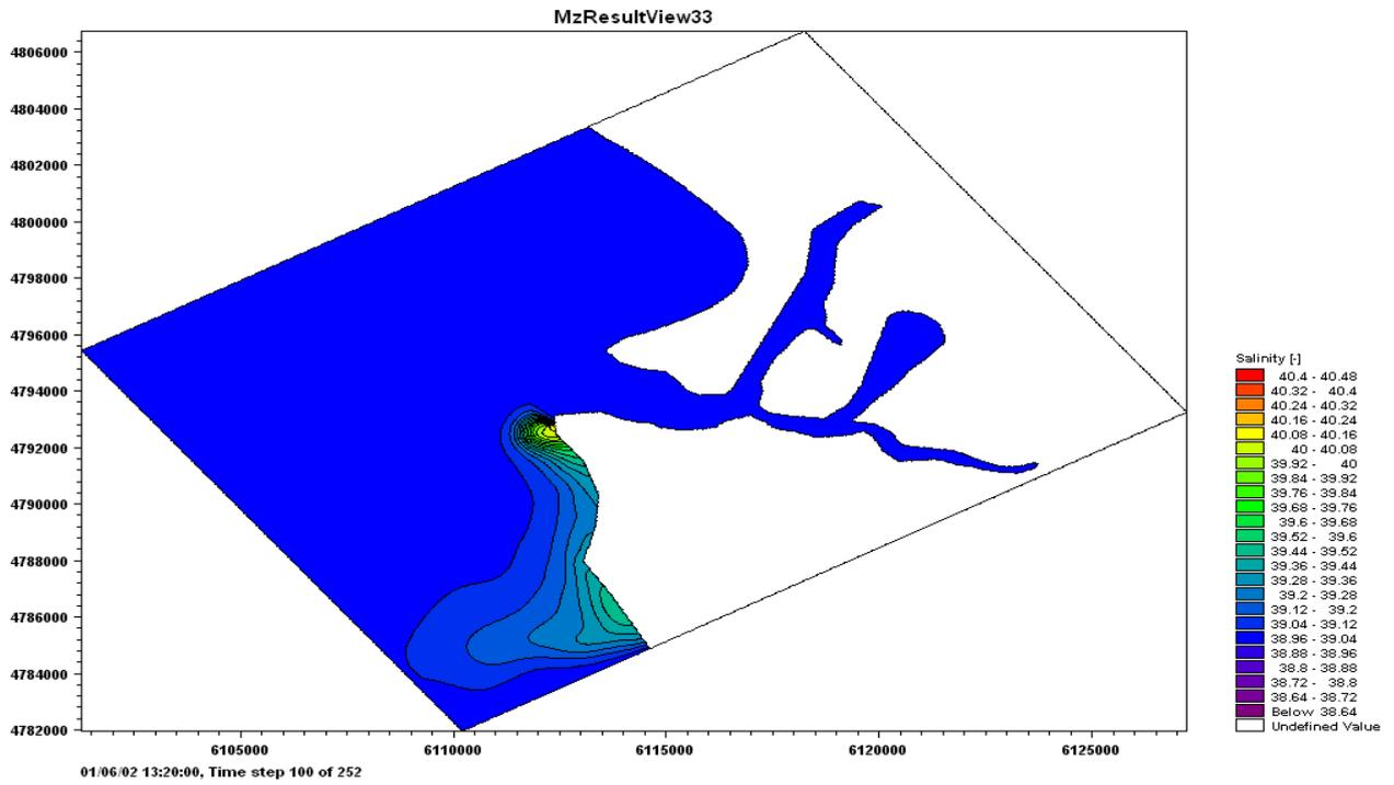
Figure 13. Simulated results of salinity at discharge, six days after the execution of the model
