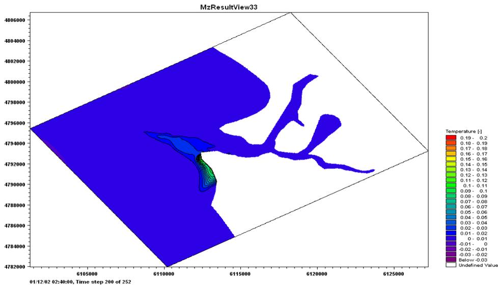
Figure 10. Simulation results of the evacuation temperature, twelve days after the execution of the model
