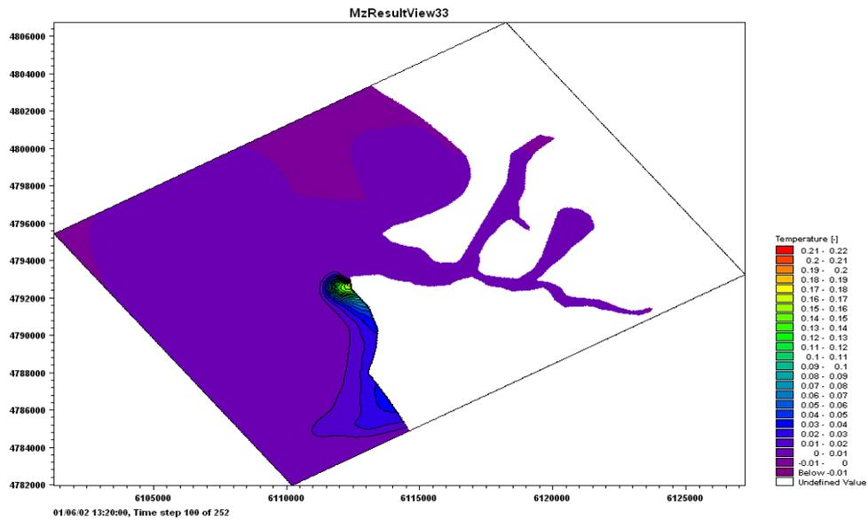
Figure 9. The simulation results of temperature at discharge, six days after the execution of the model
