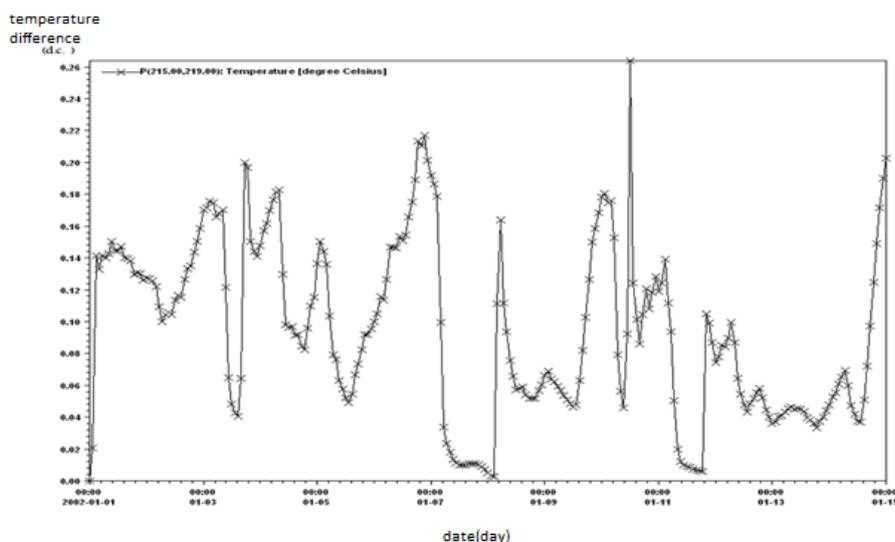
**Figure 11.** Within 200 meters of the discharge water temperature simulation results for a simulation period of 15 days from the effluent discharge scenario 1 (a distance of 477 meters and the prevailing conditions of wind and wave harvest and off-West)
