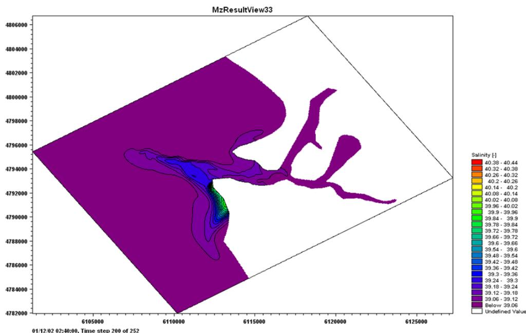
Figure 22. Simulation results in the depletion of salt, twelve days after the execution of the model
