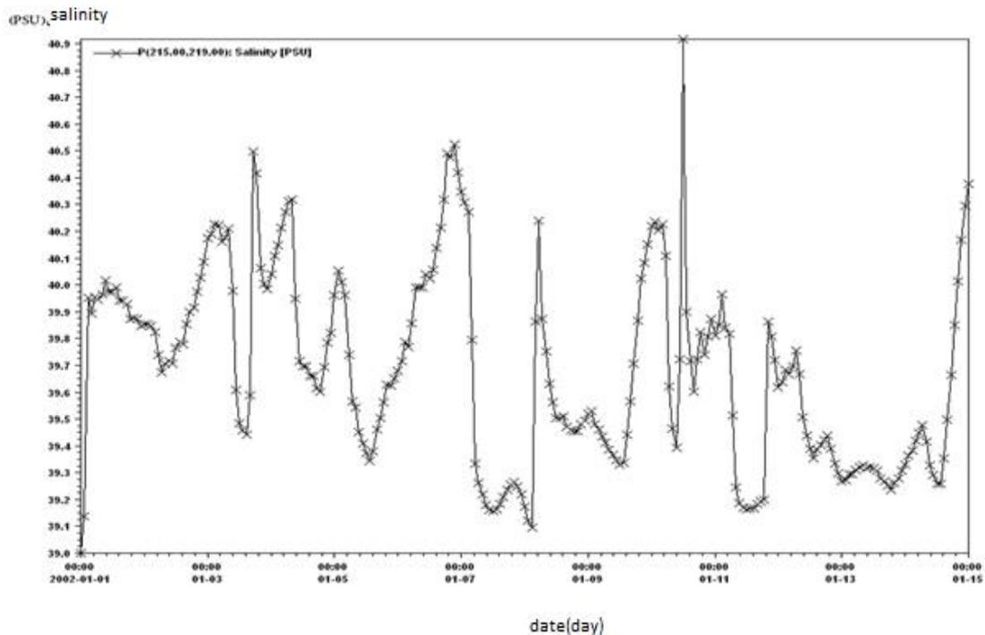
**Figure 15.**Simulation results in a radius of 200 meters of salt water discharge for a similar period 15 days from the date of discharge of effluent in scenario 1 (the distance between the harvesting and hauling 477 M and wind and wave prevailed conditions West )
