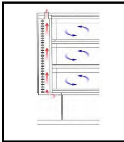
Schematic view of a Protective or partition facade
