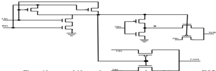
Figure10.proposal 10 transistor axis on the base of the one gate XOR
