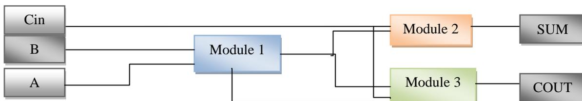
**Figure 8. full- adder diagram block with its basic models**
