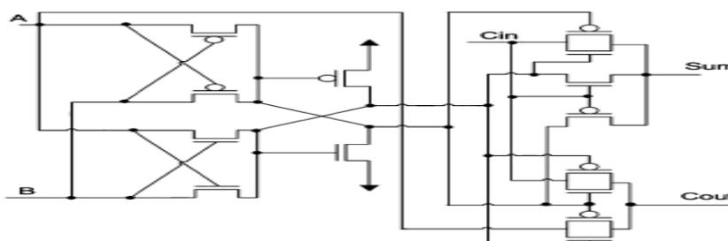
**Figure 6. 14 transistor full-adder axis**
