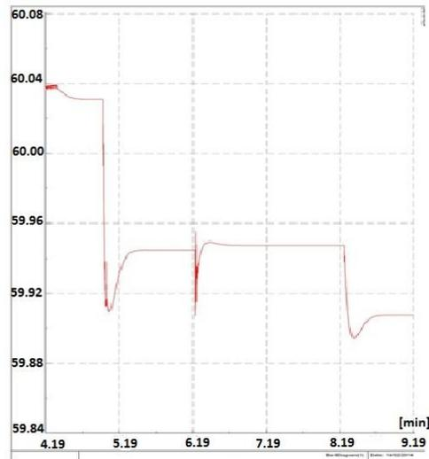
**Figure4. Frequency changes in island case, in situation of algorithm performance to use storages and other power providers**
