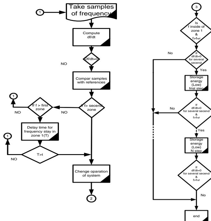
Figure2): a) the frequency sampling by this algorithm b) recognizing the zones happen with this algorithm.
