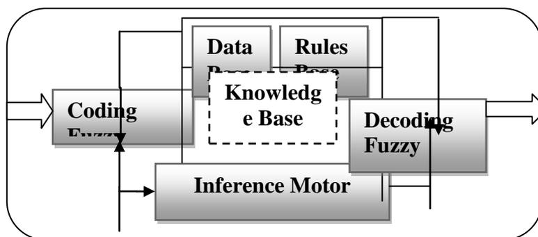
**Figure 4:** Overall view and main levels of a Fuzzy system
